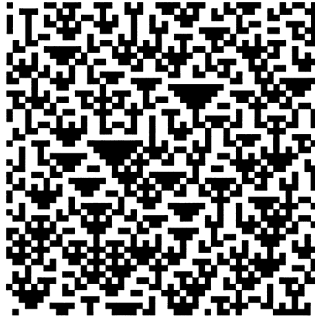
Fig. 2. Evolution of Boolean rule 90 from a random initial configuration. The black pixels correspond to the value 0, the white pixels correspond to 1.
